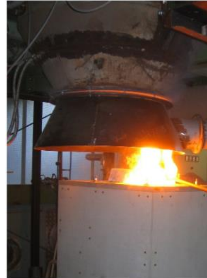
InduCarb reactor and the Flash Reactor tapping during the coupled trials
