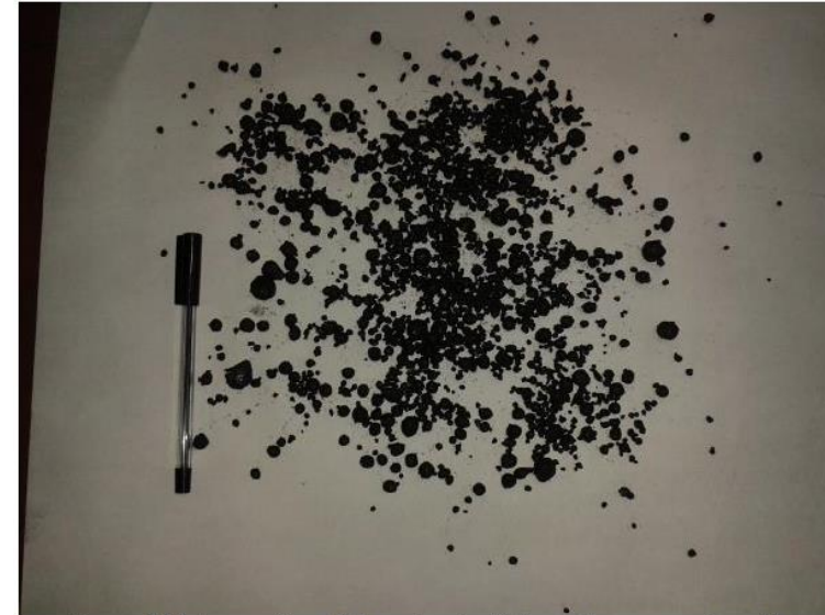
Low quality pellets produced with the mixture composition n°1.
