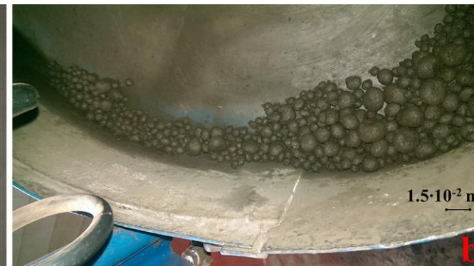
Optimized high quality pellets (BOF slag: 56÷65%; BOF sludge: 27÷36%; Lime: 1%; Cement: 7%)
